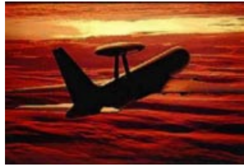
The Airborne Warning and Control System (AWACS) electronically identifies friends through the use of identification friend or foe and selective identification interrogators.
